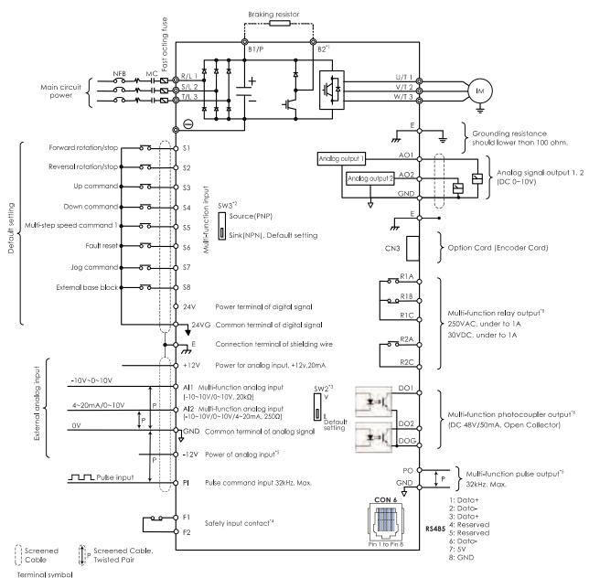
indicates main circuit o indicates control circuit
