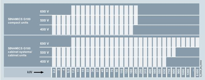
Output ranges of SINAMICS G180 (higher outputs with 400 and 500 V cabinet units available on request)
