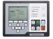
An integrated microprocessor based generator set control system providing voltage regulation, engine protection, alternator protection, operator interface and iso chronous governing. Refer to document S-1570 for more detailed information on the control. **AmpSentry** – Includes integral AmpSentry protection, which provides a full range of alternator protection functions that are matched to the alternator provided.
