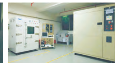
Natural convection test box (left) Cold and hot shock test box (right)
