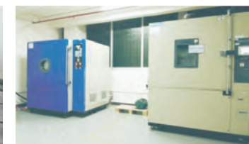
Low pressure text box (left) Constant temperature and humidity test box (right)
